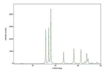
Figure 2: XRD pattern of 600°C-calcined ZnO NPs
