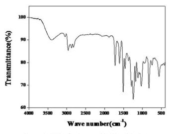
Figure 4: FTIR of polyester with 1% weight ZnO
