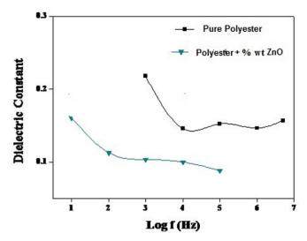
Figure 7: Frequency vs. Relative Permittivity at 100°C
